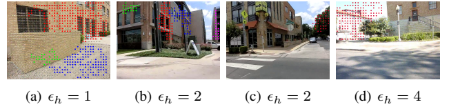
Fig. 5. Example of extracted planes. Dots with different colors indicate different extracted planes. (a-b) show all planes extracted in the frame. (c-d) show two incorrect extractions.
