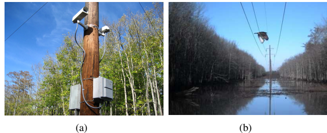
Fig. 1. Our autonomous observatory system installed along Bayou DeView, a bottomland forest near Brinkley, Arkansas. (a) The installation site. (b) A high resolution video frame of a red-tailed hawk captured by the system on Dec. 13, 2006. The red-tailed hawk has a body length of 55 cm, close in length to the IBWO.
