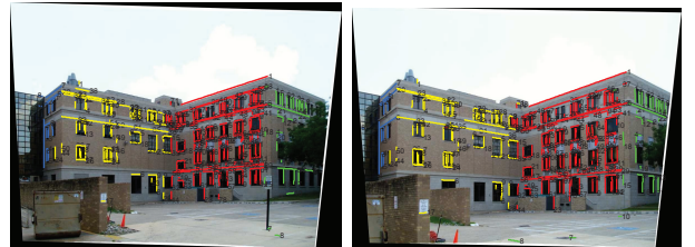
Fig. 9. Sample output for the MFG construction. We use the same color (blue yellow, red, and green) for correctly matched line segments in the same residing vertical plane.
