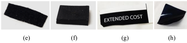
Figure 12. Photos of the eight OACTs: (a)–(d) optically-transparent targets of glass, acrylic, PET (with contour marked by dash line), PDMS with thicknesses around 1.0 mm, 1.6 mm, 0.11 mm, and 1.5 mm separately, and (e)–(h) dark thin/porous targets of fabric, foam, paper, window tint film with thicknesses around 2 mm, 8 mm, 0.1 mm, 0.06 mm separately.
