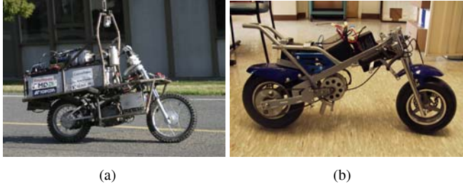
Fig. 1. (a) The Blue team autonomous motorcycle. (b) A Rutgers autonomous pocket bike.
