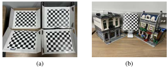
Fig. 3: (a) Example image of the training inputs for DIME-Net using the calibration rig. (b) Example image of natural object feature test setup where two LEGO buildings are the natural objects.
